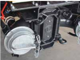
Additional feed pump
