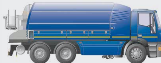
Fresh water in side-mounted water tanks in polyethylene or stainless steel
