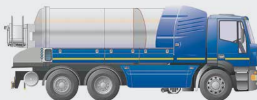
Fresh water in front section of the tank, with permanent separation from sludge tank
