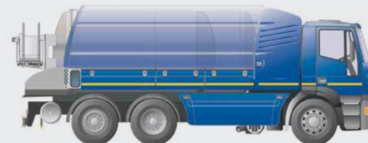
Combination of fresh water tanks at front and sides
